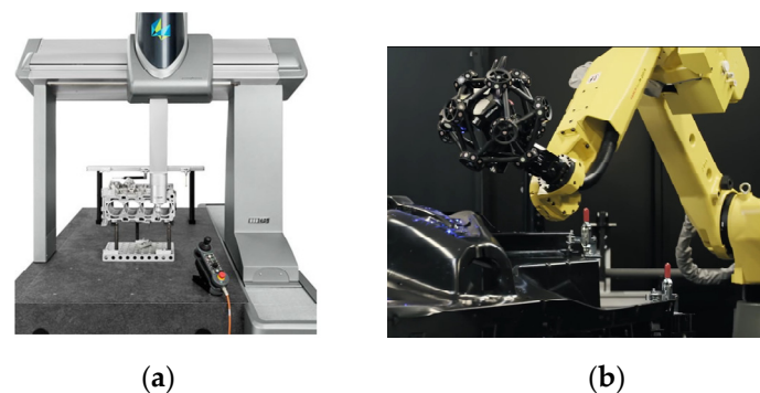
Figure 1. Two measurement methods. (a) CMM; (b) Robot optical scanning system.
