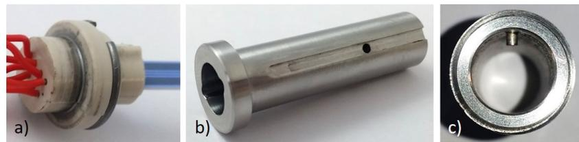
**Figure 2.** Developed sensor housing for defined horizontal sensor mounting as a modular setup: (a) two half shells (PEEK) clamp the ceramic sensor substrate together with electric contact wires; (b) a stainless steel adapter fits the flange (c), which is welded to the flue pipe of the chimney.
