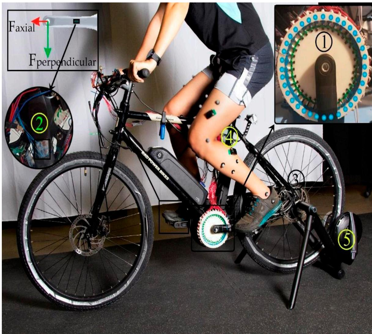
**Figure 1.** The APAD consisted of a crank position sensing system (1) and force sensor (2), BLDC rear hub motor (3), and a controller (4). The APAD was mounted on a trainer (5) for testing in the motion capture lab. The crank tracking unit consisted of 36 hall sensors on the 3D-printed fixture. The strain gauges-based force sensor measured the crank's perpendicular force. The ID number of each hall sensor to the controller is pictured along the circumference of the unit.
