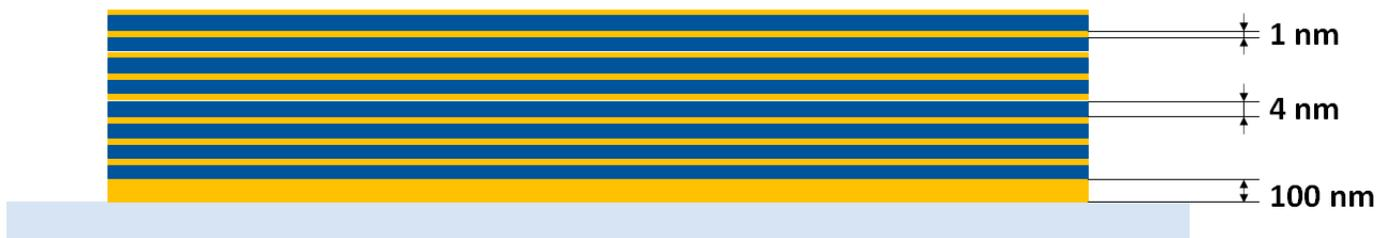
**Figure 1.** Scheme and dimensions of the structure in the current to plane configuration.
