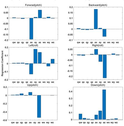
**Figure 7.** Result of sensitivity analysis on gesture mode movements. In particular, gestures such as forward, backward, up, and down were found to perform numerous pitch motions. Left and right gestures were known to perform roll actions primarily. According to the results, acceleration of x, y, z and angular velocity of y and z were determined to be key parameters in common.
