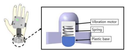
Figure 3. Structure of vibrotactile stimulator.
