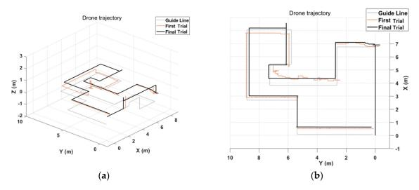
**Figure 13.** Example of drone flight trajectory with gesture mode. Gray line is guideline, dotted line represents drone trajectory of first trial, and black line is last trial. (a) Isometric view can be found altitude control using gestures. (b) Top view of drone trajectory can be figured out drone movements on x-y dimension. While first trial is low-accuracy and the trajectory is unstable, last trial is high-accuracy and confirms that the trajectory appeared similar to the guideline.
