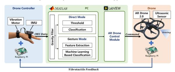
**Figure 2.** System configuration of wearable drone interface comprises a drone controller, hand gesture recognition and drone control module in PC, and drone.
