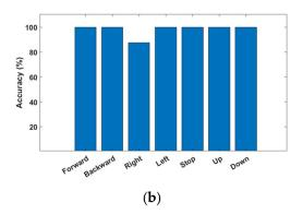
**Figure 19.** Accuracy of real drone control. (a) Average accuracy of direct mode is about 96%, which is about 2.6% lower than the simulation. (b) Average accuracy of gesture mode is about 98%, which is about 1.4% higher than the simulation.
