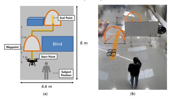
**Figure 20.** Flight experiment for vibrotactile feedback with gesture mode. (a) Schematic diagram comprising visual obstruction, drone, passing gates, obstacle, and guideline. (b) Based on the scheme, flight experiment was set up.
