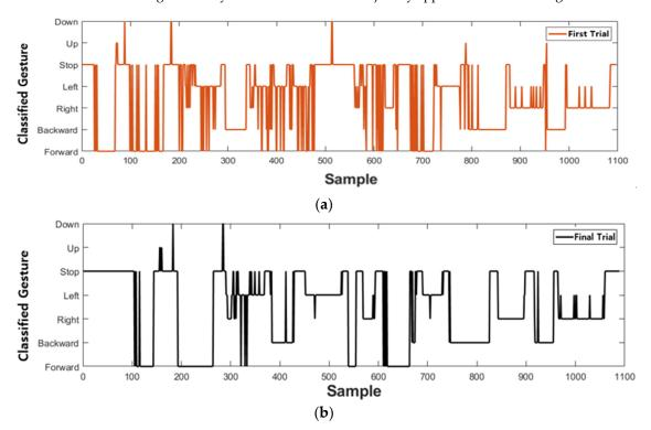
**Figure 14.** Frequency of gesture changes during trial duration with gesture mode. (a) Classified gesture changes at first mission. (b) Classified gesture changes at last trial, which shows less change than first trial.
