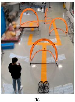
**Figure 18.** Experiment scenario with gesture-based drone control. (a) Schematic diagram for experiment. The yellow guideline was installed for reference of drone trajectory. The user walked within gray dotted lines to secure the view. (b) Experiment environment based on schematic was set indoors for safe operation.
