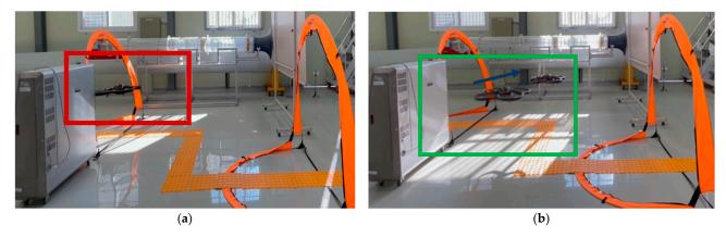
**Figure 21.** Result of vibrotactile feedback. (a) Drone could not avoid the collision in front. Owing to the lack of visual information for the obstacle, the mission failed. (b) Drone flew successfully through gates, and distance to the obstacle was maintained using vibrotactile feedback.
