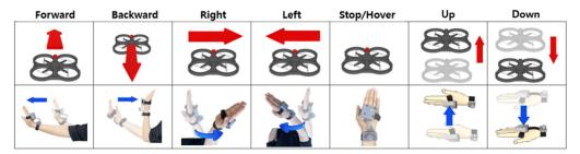
**Figure 5.** Definition of gesture mode. Gesture mode can control the direction of drone with natural hand motion.
