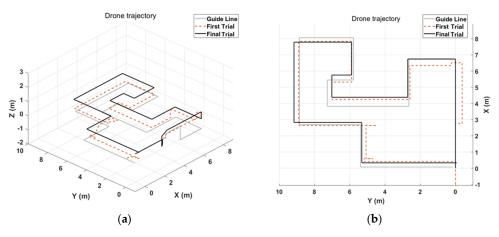
**Figure 10.** Example of drone flight trajectory with direct mode. Gray line is guideline, dotted line is trajectory of first trial, and black line is trajectory of last trial. Comparing the trajectory between first and last trials, the last one is a more stable shape. (a) Isometric view of drone trajectory can be found by adjusting drone altitude. (b) Top view of drone trajectory can be determined by behavior of drone according to the user on the x-y dimension.
