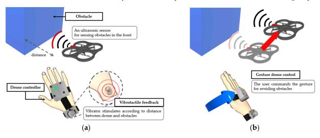
**Figure 1.** Concept of the proposed controller with vibrotactile feedback and gesture-based drone control. (a) Obstacle is detected in front of the drone, and the vibrator is stimulated. (b) Gesture of right direction is performed to avoid obstacle using gesture control.
