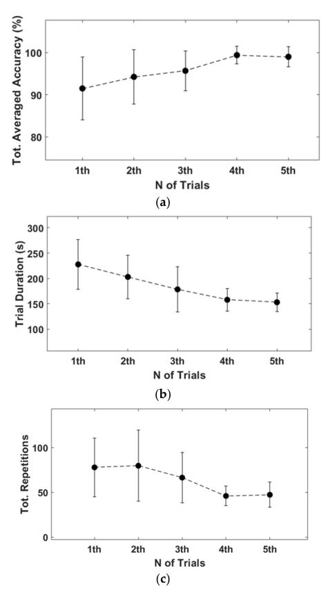
**Figure 12.** Results of direct mode simulation (mean  $\pm$  SD). (a) Total average accuracy of each trial. First trial is 91.5  $\pm$ 7.4%, and last trial is 99  $\pm$  2.4%. (b) Average trial duration. First trial is 227.7  $\pm$  48.7 s, and last trial is 153.0  $\pm$  18.1 s. (c) Total repetitions of gestures. First trial is 77.8  $\pm$  32.8, and last trial is 47.2  $\pm$  14.0.
