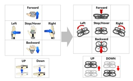
**Figure 4.** Definition of direct mode. It can directly control the drone's posture and speed according to inclination and up/down of hand.
