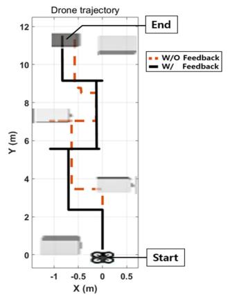
**Figure 17.** Example of drone flight trajectories with and without vibrotactile conditions. When the vibrotactile feedback did not work, the drone crashed into boxes because of lack of visual feedback (dashed line). With vibrotactile feedback, the drone achieved the mission of avoiding obstacles (black line).
