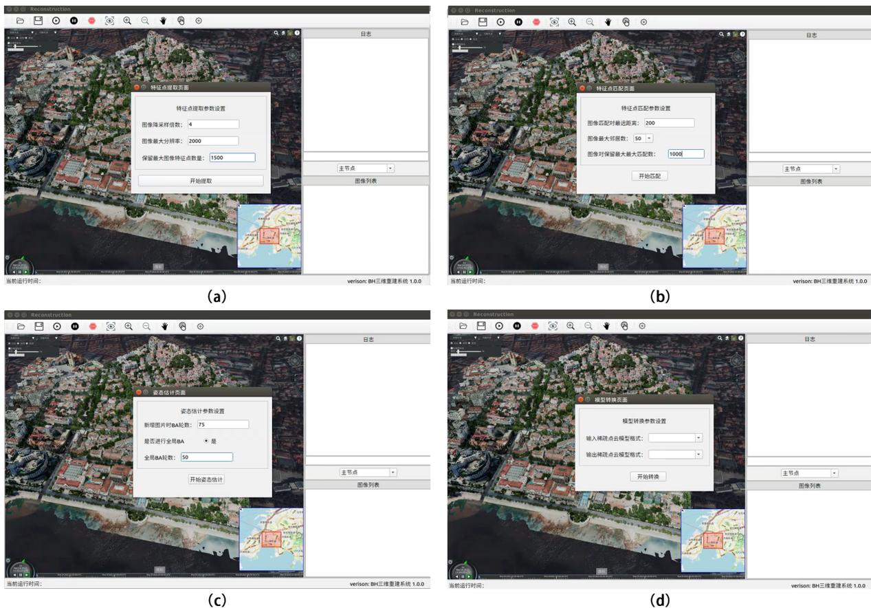
**Figure 10.** In expert mode (professional parameter setting), the sparse point-cloud 3D-reconstruction example is completed by setting parameters in four steps: (a) feature-point extraction, (b) feature-point matching, (c) bundle adjustment and (d) model format conversion.
