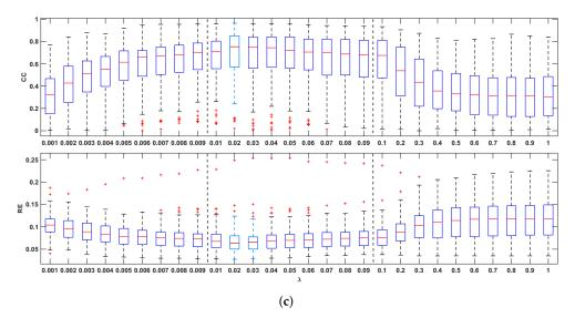
**Figure 2.** Boxplots summarizing the influence of the regularization parameter on reconstructed electrograms ((a), two top panels), activation times ((b), two middle panels), and recovery times ((c) two bottom panels). The best results are indicated with light blue boxplots. Whiskers range from the end of the interquartile range to the furthest observation within the whisker length that is not considered an outlier.
