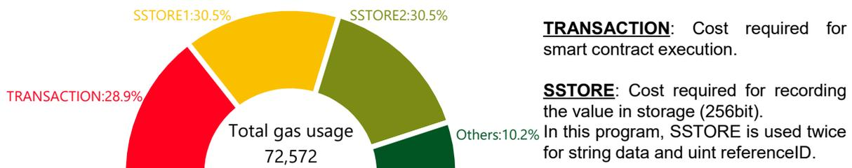
Figure 6. Breakdown of gas usage in a transaction.
