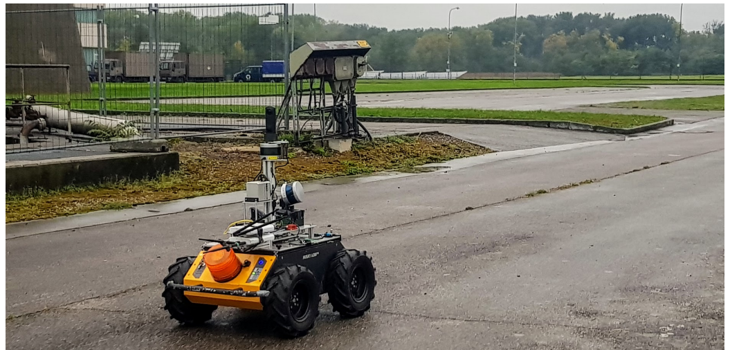
Figure 8. Robotic platform equipped with multiple mapping systems. This robot was used for the evaluation of the proposed contribution. The robot provided two 3D data streams for further comparison.
