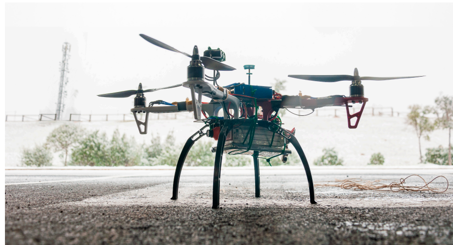
Figure 4. UAV built from scratch to meet the formulated requirements. Note the MDAS subsystem added to the bottom part.
