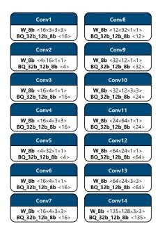
Figure 3. Model compression through data quantization on convolutions.
