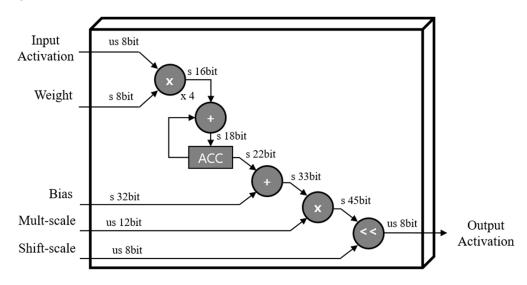
**Figure 7.** Convolution operation in PE:  $1 \times 1$  case.
