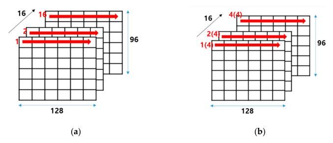
**Figure 9.** Overall process flow: (a) in ofmap write operation on on-chip memory at conv1 layer; (b) in ifmap read operation on on-chip memory at maxpool layer, and maxpool operation on maxpool unit.
