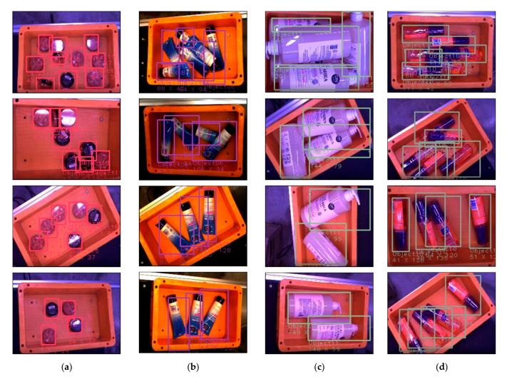
**Figure 10.** Qualitative evaluation of the performance on object detection of the proposed model. There are different objects in horizontal, and different number of objects and angle in vertical: (a) small objects with red and black color; (b) middle size of objects with blue, white, and black color; (c) big size of objects with white color; (d) middle size of objects with pink and purple color.
