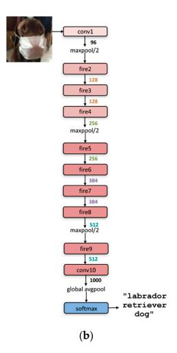
**Figure 1.** SqueezeNet architecture [21]: (a) micro-architectural view: fire module structure in the SqueezeNet; (b) macro-architectural view: SqueezeNet comprises a series of fire modules.
