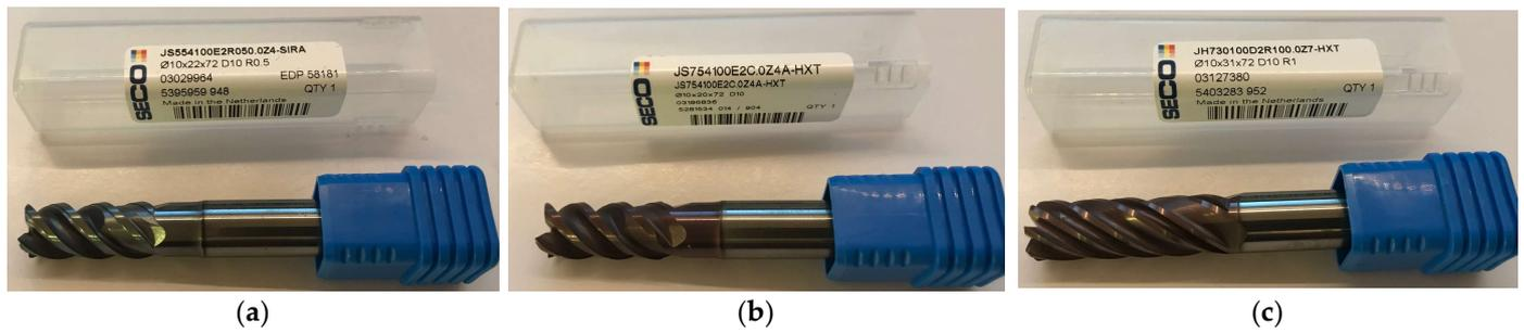
**Figure 2.** Monolithic milling cutters used to prepare samples: (a) Tool 1: JS554100E2R050.0Z4-SIRA; (b) Tool 2: JS754100E2C.0Z4A-HXT; (c) Tool 3: JH730100D2R100.0Z7-HXT.
