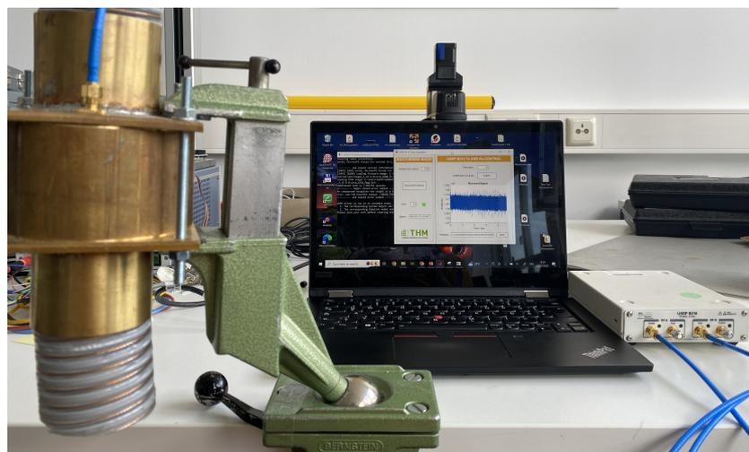
(b) Developed mass flow sensor connected to a PC via USRP B210.
