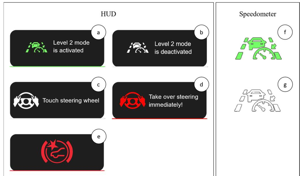
**Figure 5.** System information in HUD: (a) Partially automated driving system activated; (b) Partially automated driving system deactivated; (c) Touch steering wheel; (d) Take over steering immediately!; (e) Collision warning. System information in speedometer: (f) Partially automated driving system active; (g) Partially automated driving system inactive. Messages are according to Volkswagen’s design [47].
