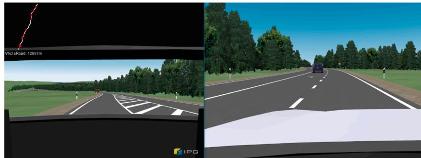
**Figure 4.** View from rear-view mirror with truck approaching on the left and view through windscreen shortly before phantom braking on the right.
