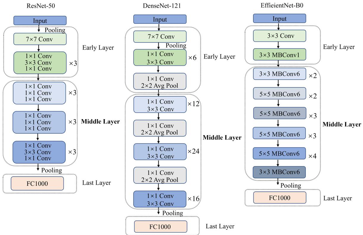
**Figure 3.** The structures of the early, midlevel, and last layers in different CNNs.
