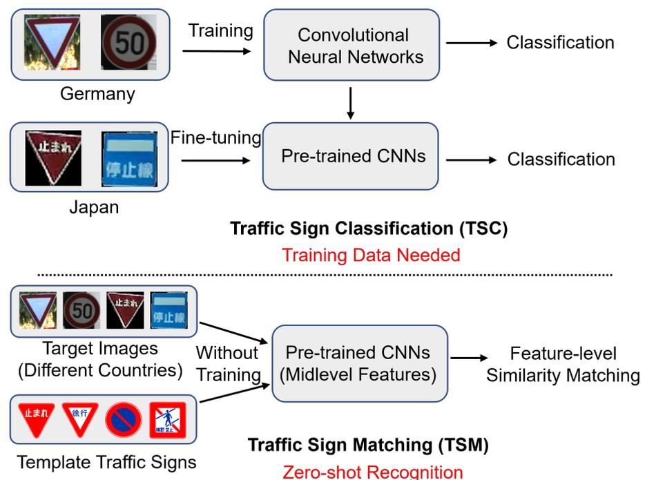
**Figure 1.** Concept of the proposed zero-shot traffic sign recognition method. This method can perform traffic sign recognition for different countries without collecting training data. Common traffic sign templates for each country can be used.
