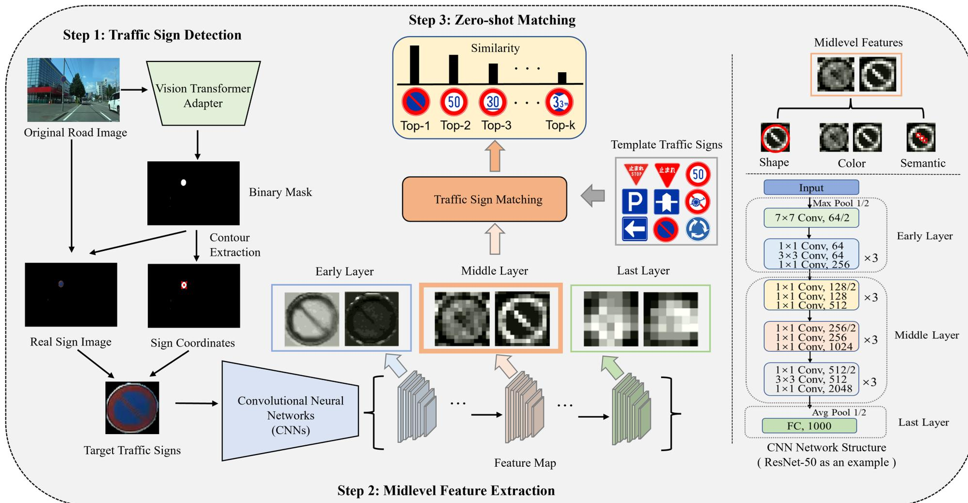
**Figure 2.** Overview of the proposed traffic sign recognition method. We first extract the target traffic signs from the road images based on ViT-Adapter. We then use the midlevel features of CNNs to perform TSM.
