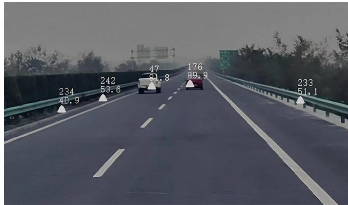
**Figure 12.** The radar is used to detect target projections in the image.
