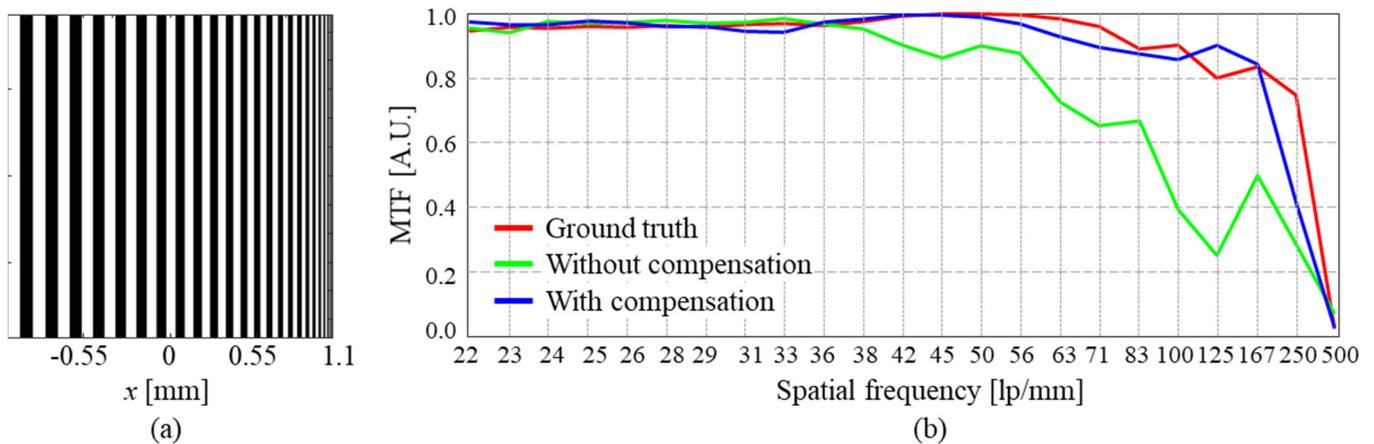
**Figure 10.** Resolution analysis of the SA-DHM. (a) Resolution target. (b) MTF chart with and without compensating aberration by using the proposed DNN.
