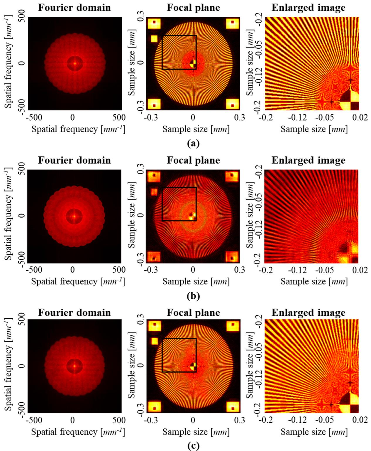
**Figure 11.** SA-DHM reconstruction results with the spoke resolution chart, and their enlarged images. (a) Ground truth and (b) reconstruction without compensating aberration. (c) Reconstructions with compensating the aberration.
