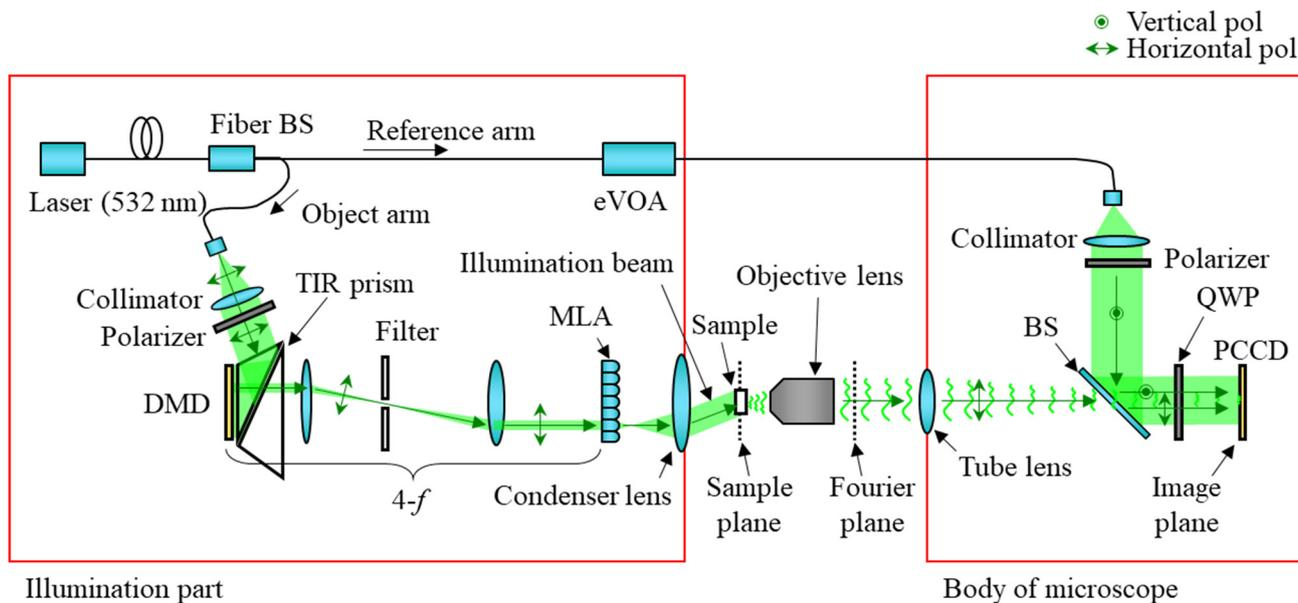
Figure 1. The structure of a synthetic aperture digital holographic microscope.
