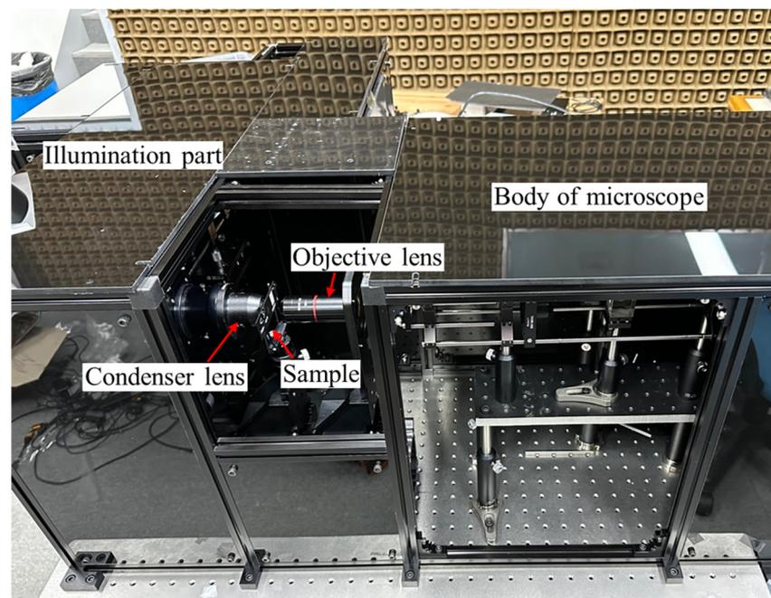
**Figure 2.** Implemented synthetic aperture digital holographic microscope.
