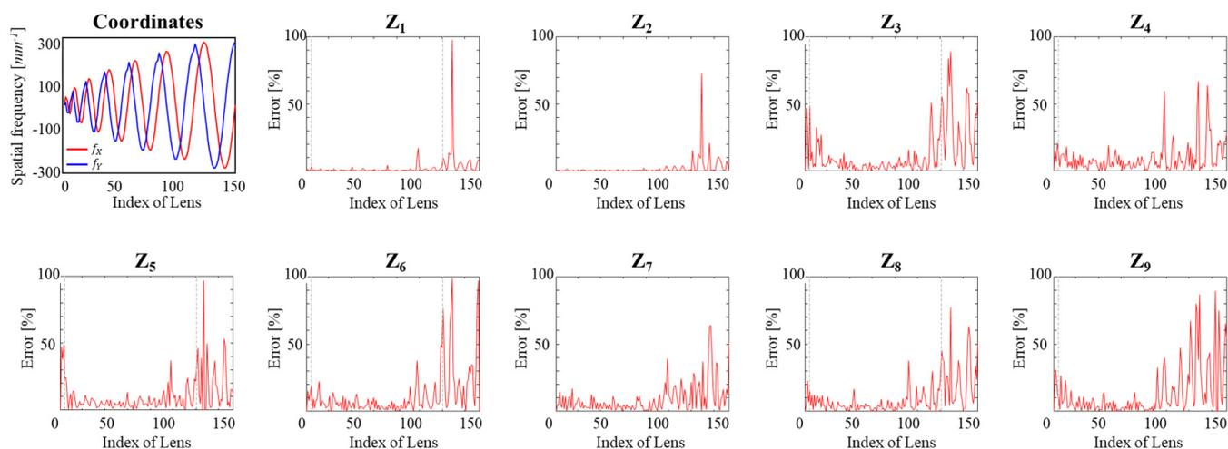
**Figure 8.** Estimation errors in nine Zernike coefficients of aberration of illumination beams.
