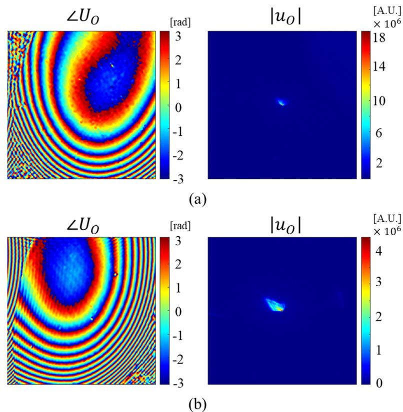
**Figure 3.** Experimental measurements of intensity phase profiles in focal plane and in Fourier domain. The measurements from the illumination beams are (a)  $\vec{k}_i = (122.1, -163.6, 11,808.3)$  and (b)  $(187.6, -164.6, 11,807.9)$ .
