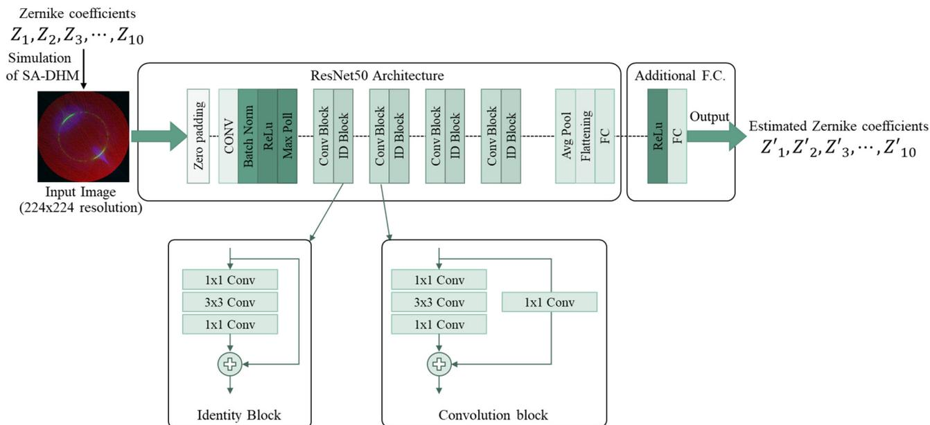
**Figure 4.** Structure of ResNet50 for Zernike coefficients. The ResNet consists of identity blocks and convolution blocks, and a fully connected layer is added to estimate the ten lowest Zernike coefficients.
