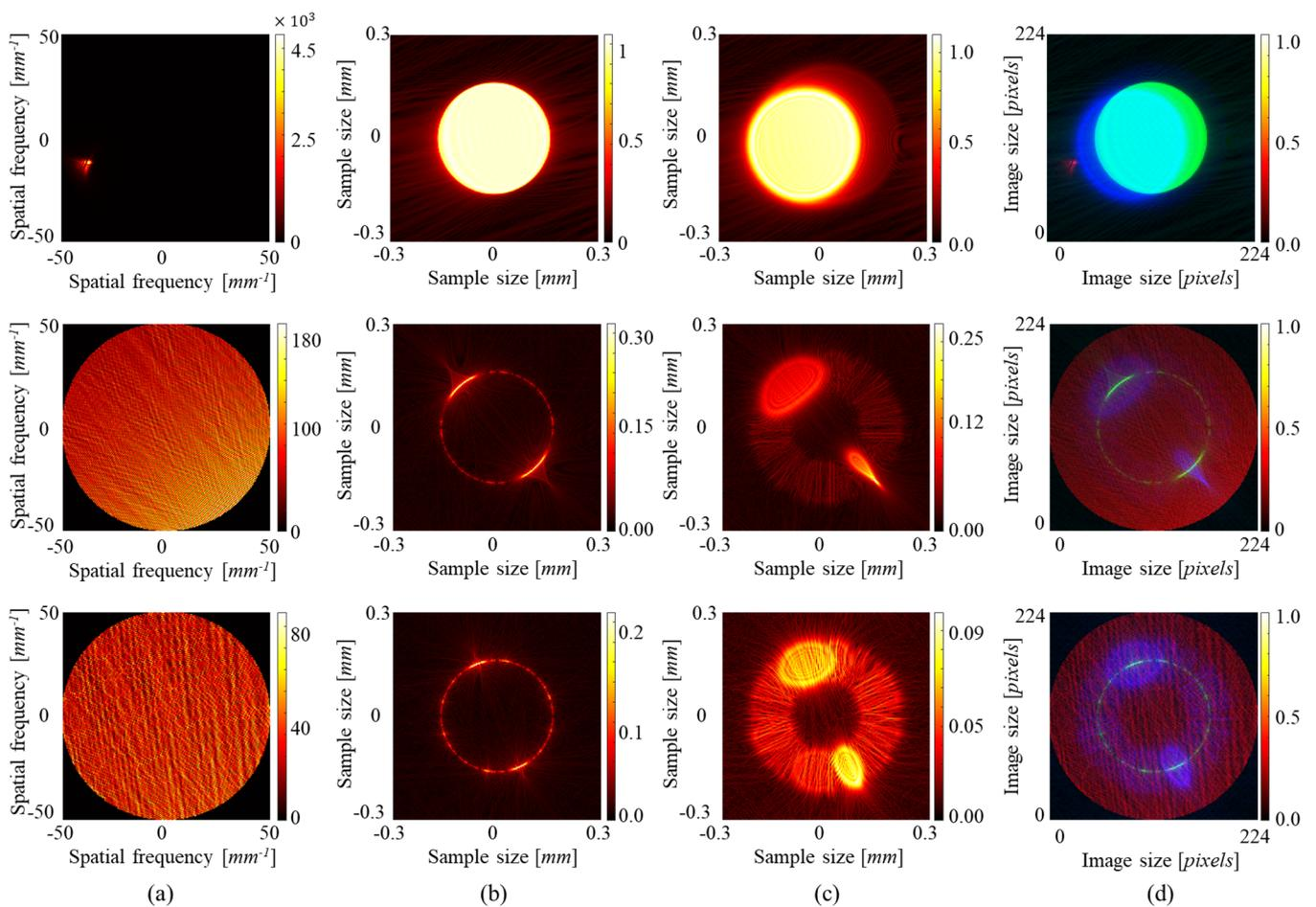
**Figure 6.** Examples of the training data. The intensity patterns on (a) the Fourier domain, (b) the focal plane, and (c) the out-of-focus plane. (d) They are, respectively, occupied in R, G, B channels for training data. The pictures on the first line were numerically generated in the bright field condition and the others were numerically generated in the dark field condition.
