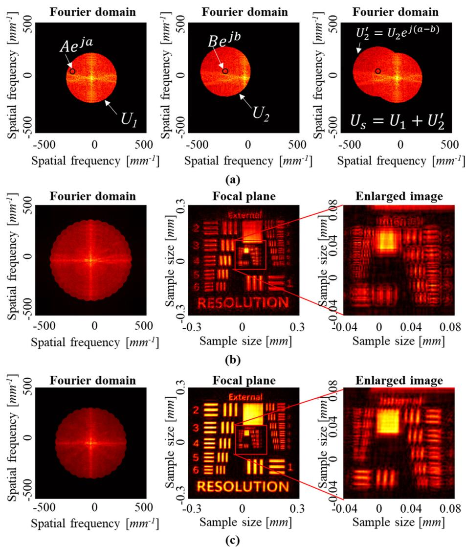
**Figure 12.** Piston phase matching and numerical reconstruction results. (a) Piston phase matching at a specific point in overlapped region. Numerical reconstruction results (b) without and (c) with piston phase matching.
