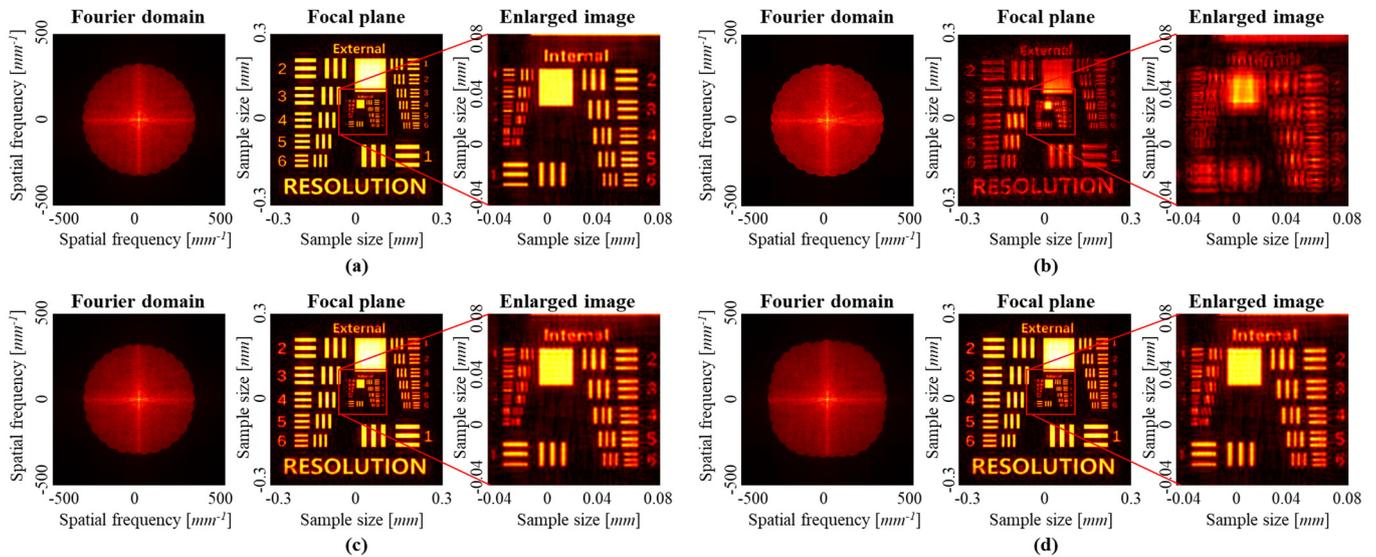
**Figure 9.** SA-DHM reconstruction results of synthesized intensity profiles in Fourier domain, reconstruction images in focal plane, and their enlarged images. (a) Ground truth and (b) reconstruction without compensating aberration. Reconstructions with compensating the aberration (c) within and (d) outside the range of training data.
