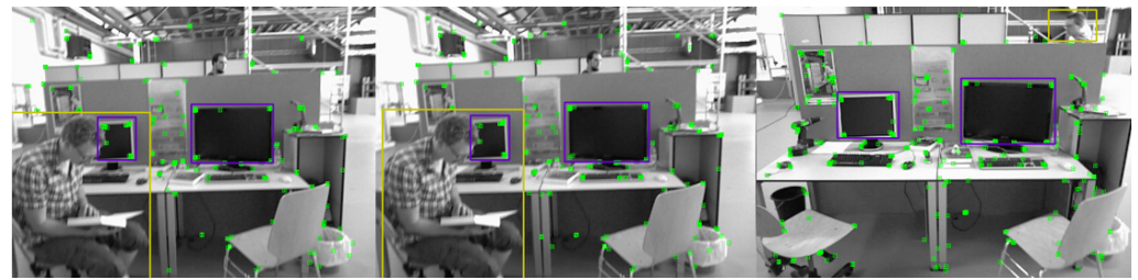
Figure 10. High Dynamic Objects Gain Higher Attention.(When a highly dynamic object is in a static position in space and moves further away from the camera, it can still be better captured by a lightweight target detection network) High dynamic objects are in the yellow box and low dynamic objects are in the purple box.
