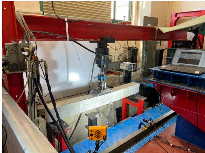
**Figure 4.** DIC system set-up.
