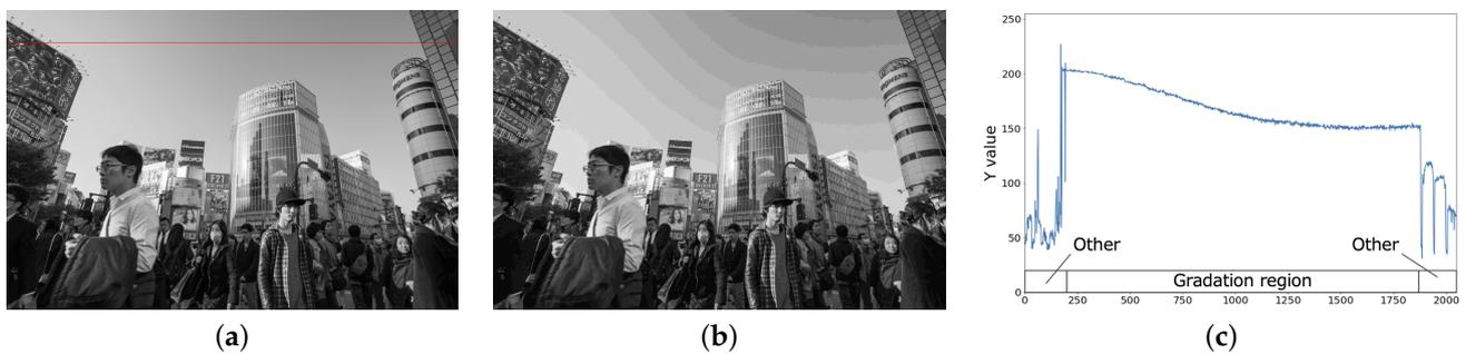
**Figure 6.** Y channels of an image containing gradient region. (a) Original image; (b) JPEG image; (c) Luminance values on red line.
