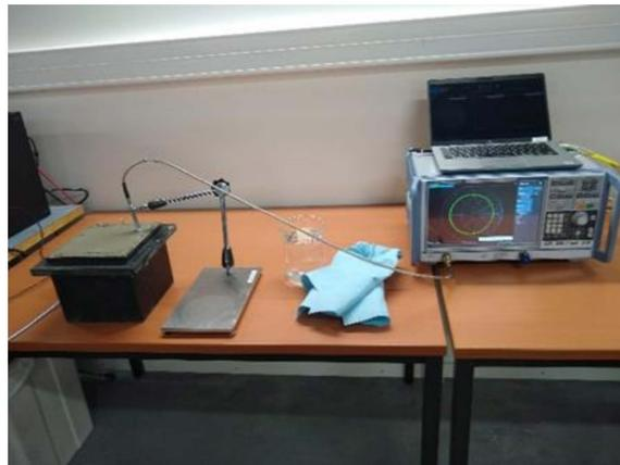
**Figure 3.** The dielectric measurement setup with the Speag DAK connected to the R&S VNA. In the picture, the concrete cube is still in its mold.
