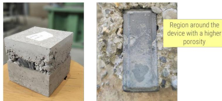
**Figure 9.** Poor distribution and compaction of concrete around the hardware device.
