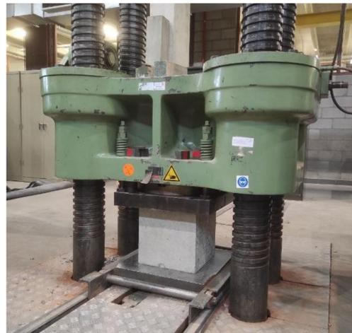
**Figure 7.** Testing machine used for assessing the compressive strength of the cubes.
