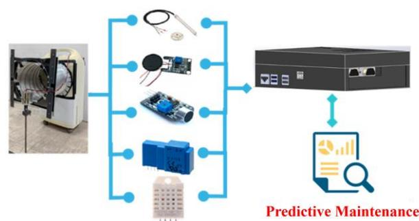
**Figure 9.** Experimental scheme for integration test.
