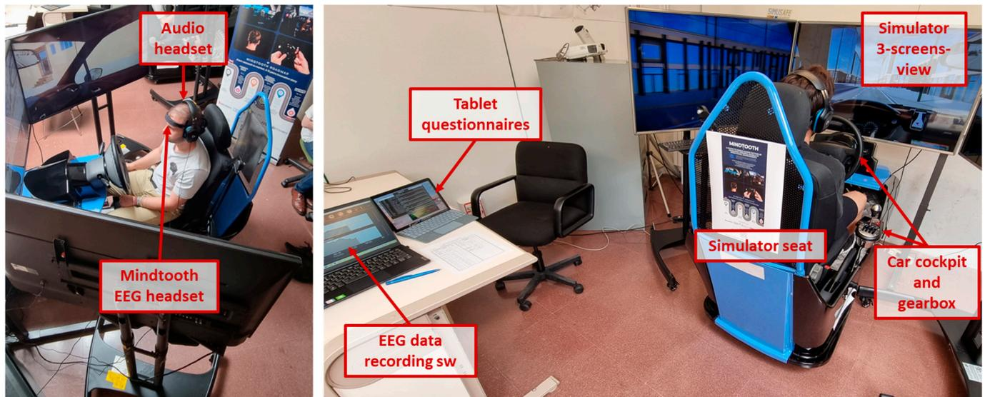
**Figure 2.** Experimental room at the University of Burgos with the two car simulators. The participant, seated in the simulator, wears the audio headset and the Mindtooth EEG system. The EEG data were collected by means of the Mindtooth proprietary recording software (v.5.22). The simulator consists of a real car seat, with a coherent cockpit, the steering wheel, and the gearbox. A tablet was used to provide self-assessment questionnaires digitally.
