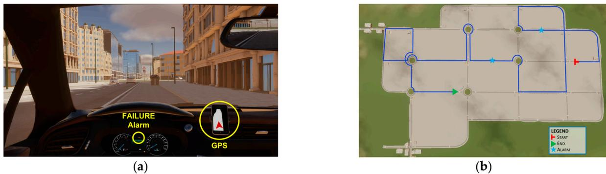
**Figure 3.** On the left (a), a screenshot of the simulated driving scenario within the urban environment: highlighted the failure alarm light on the dashboard and the GPS system indicating the route to follow. On the right (b), the route (in blue) designed for the adaptation task with the position of the failure events ('ALARM').
