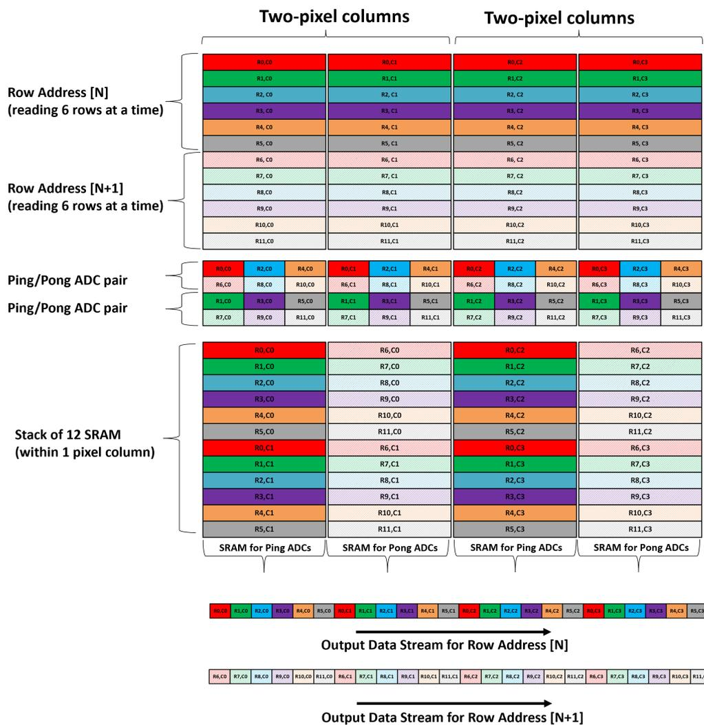
Figure 6. Data aggregation and readout order for single-gain mode.
