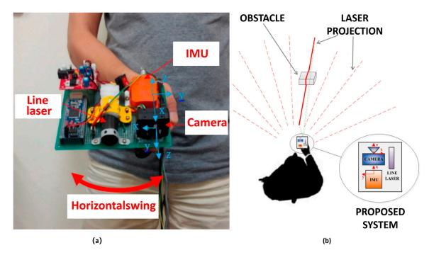
**Figure 5.** (a) Smart cane composed of camera, linear laser and IMU; (b) Working diagram of the smart cane system [74].
