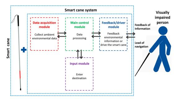
Figure 1. Structure diagram of smart cane.
