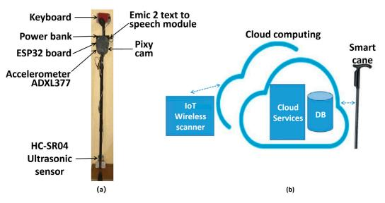
Figure 4. (a) The components of the Smart Cane; (b) The system structure of smart cane [55].
