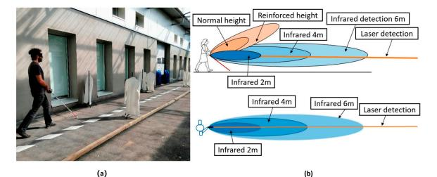
**Figure 2.** (a) A visually impaired holding the Tom Pouce III laser smart cane; (b) the detection range of the smart cane [37].
