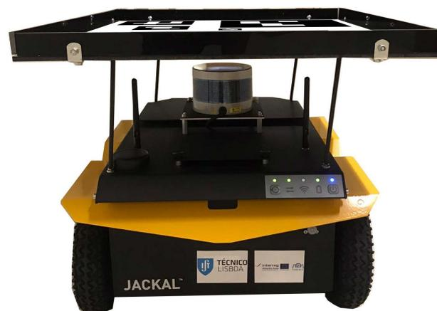
**Figure 2.** Jackal mobile robot with landing platform and marker pattern on top.
