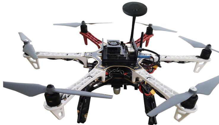
**Figure 1.** Unmanned aerial vehicle based on a DJI F550 hexacopter.
