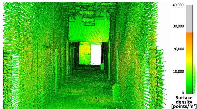
Figure 11. Point cloud density—tilting lidar.
