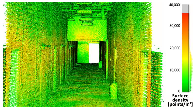
Figure 10. Point cloud density— rotating lidar.
