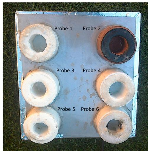
**Figure 2.** Anti-biofouling techniques probes. Probe 1: ABS material; Probe 2: PLA with copper filament; Probe 3: PDMS coating; Probe 4: PLA material; Probe 5: epoxy coating; Probe 6: chlorine production.
