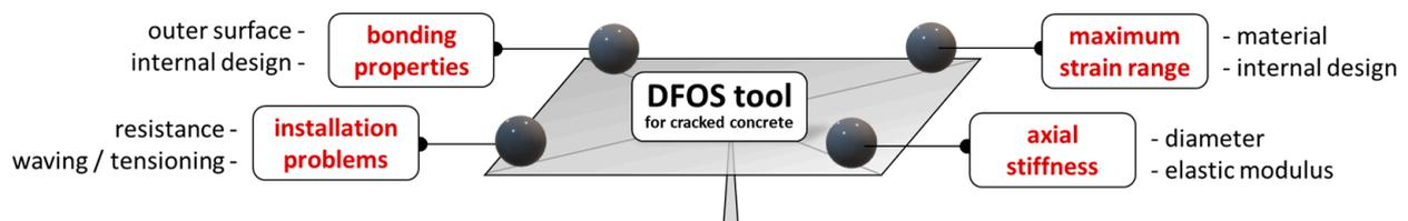
**Figure 32.** Issues that should be addressed while selecting the appropriate DFOS tool for monitoring the cracked concrete structures.
