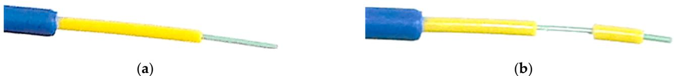
**Figure 10.** Graphical presentation of possible slippage between the layers: (a) stripped three-layer cable; (b) the piece of intermediate layer slipped against the internal layer.
