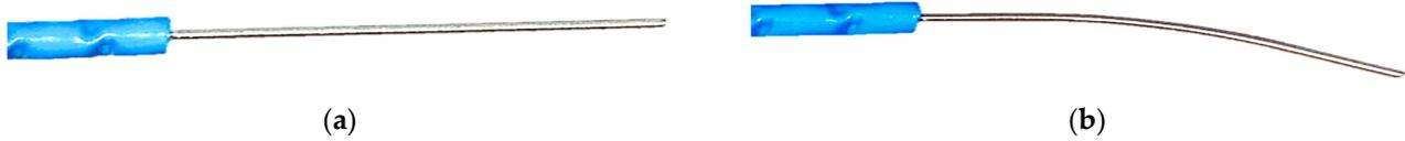
**Figure 11.** Layered cable with steel strengthening insert: (a) before the deformation; (b) after the permanent (plastic) deformation.
