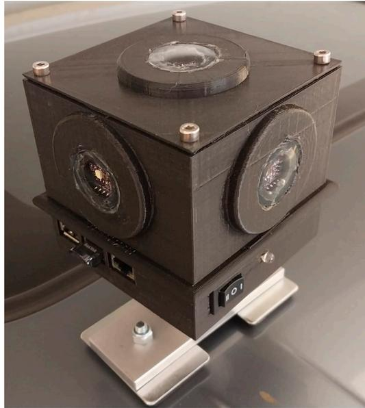
**Figure 4.** The LANcube v2 (LAN3V2) as mounted on the roof a car.
