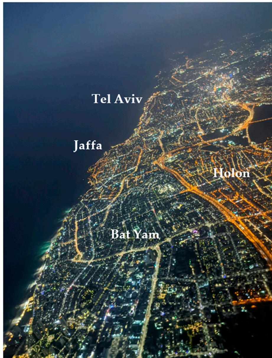
**Figure 11.** Aerial night-time photo acquired on 28 October 2022, contrasting the night-time lights of Bat Yam (mostly LED street lights) and Holon (mostly HPS street lights). Note the spatial variability in night-time light brightness and color. Photo taken by Shahar Har'el.
