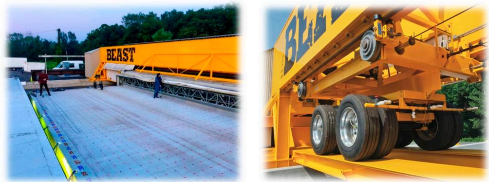
**Figure 18.** The bridge deck in the BEAST facility (left) and the dual-axle carriage (right).
