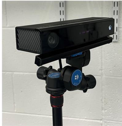
**Figure 11.** Interfering secondary ToF sensor mounted to a tripod using the Benro 3-Way Geared Head.
