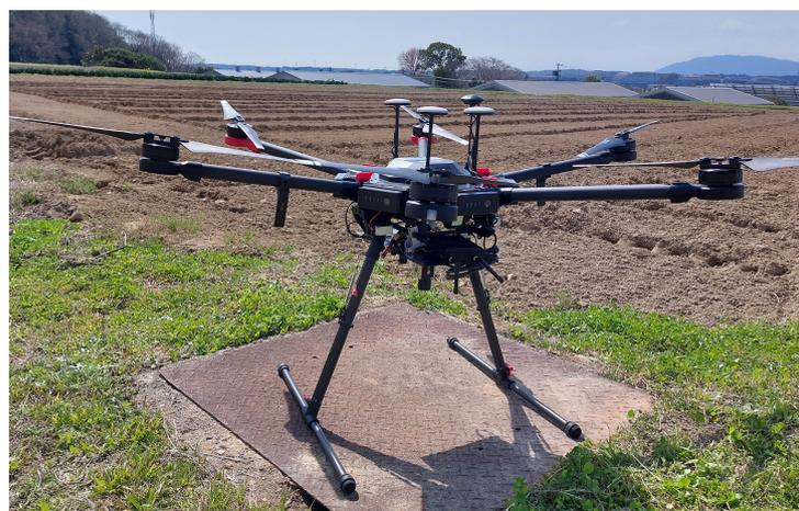
**Figure 2.** The DJI M600 Pro drone with mounted camera.
