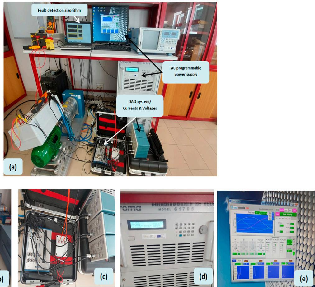
**Figure 2.** (a) Experimental test bench; (b) the fault detection algorithm; (c) the acquisition system; (d) AC programmable power supply; (e) AC power supply platform.
