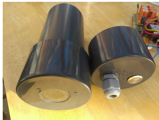
Figure 2. A photograph of the capture device with top part removed showing the camera window and power supply and switch.
