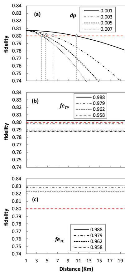
Figure 8. QP2MP quantum technologies performance comparison; Performance of QP2MP-DT (a); Performance of QP2MP-TP (b); Performance of QP2MP-TC (c).
