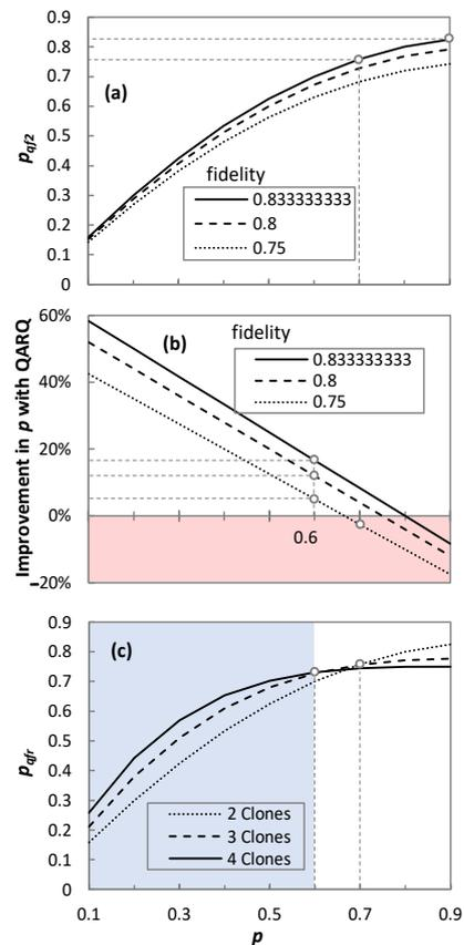
**Figure 7.** Probability of successful transmission with and without QARQ;  $p_{qfr}$  curve at different fidelities of qubit (a); Improvement in  $p$  with QARQ at different fidelities of qubit (b);  $p_{qfr}$  curve for different no. of clones (c).
