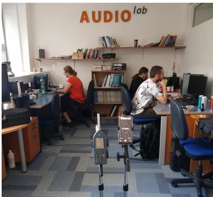
**Figure 3.** The measurement setup for background noise recording. Norsonic Nor140 on the left side and Xiaomi Redmi Note 10 Pro on the right side. Case office with carpet and people working on PCs.
