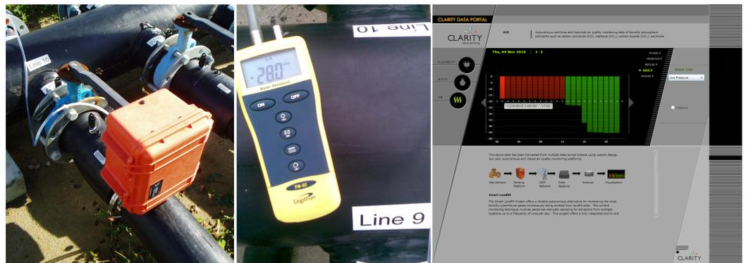
**Figure 3.** Captured photos of the deployed sensing system (left) and a pressure spot check with a reference instrument (middle). Screen grab of the sensor portal web application showing a portion of the captured pressure data (right).
