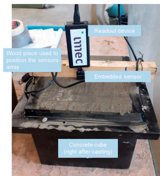
**Figure 3.** Experimental setup: sensor installation in concrete with readout for data acquisition.
