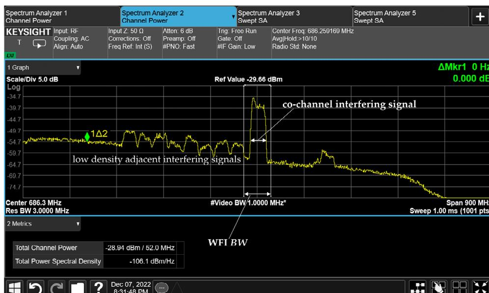
Figure 8. Power spectrum of the interference,  $f_c = 8308$  MHz.
