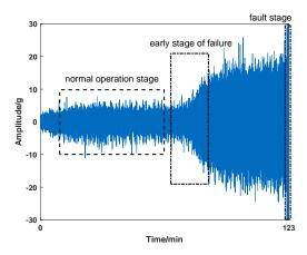
Figure 1. The three stages of equipment running status.
