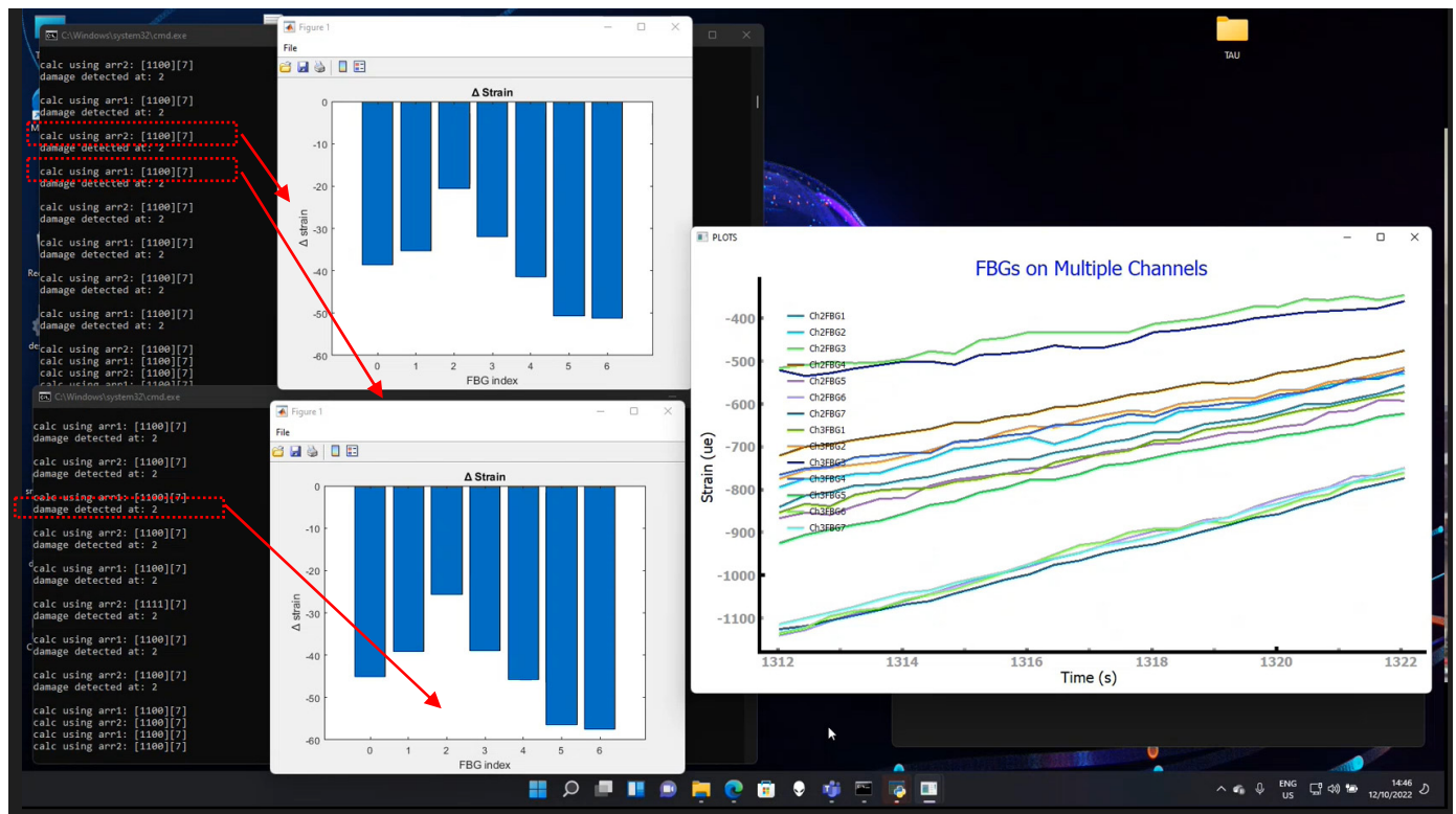
Figure 10. Screenshot of the SHM module running in real-time mode. Red box indicates the channel (arr1 and arr2) with the corresponding bar plot and the readout (damage detected at sensor number 2).
