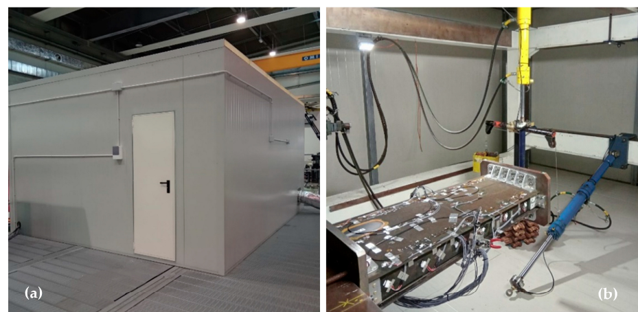
Figure 3. Actual test configuration: (a) left picture reports the climatic chamber specifically designed to host the test rig; and (b) right picture reports the bending actuator installed on the test article, while the compression actuator is detached.
