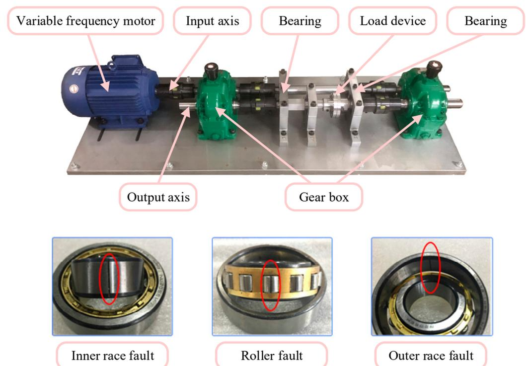
**Figure 5.** Time-varying speed bearing fault experimental bench and faulty bearing.
