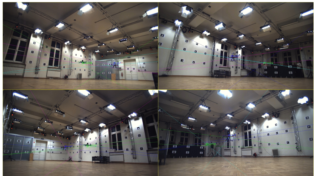
Figure 1. Multi-camera drone registration. Determined bounding boxes and epipolar lines are visualized.
