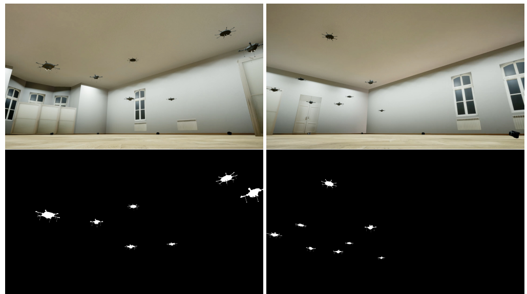
Figure 6. AirSim simulation with eight flying drones. Two selected video frames ( at the top ) with corresponding drone masks ( at the bottom ), were obtained at the same time from different cameras.
