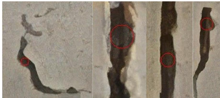
**Figure 12.** Visual annotation of maximum crack width in small-size sub-images.
