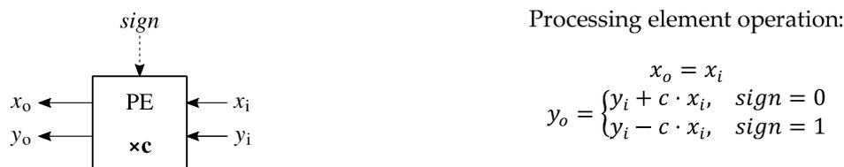
**Figure 4.** The function of a processing element (PE) used in the systolic array [33].
