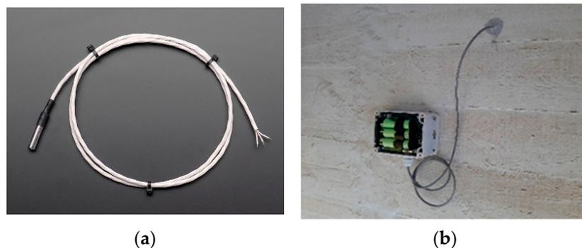
**Figure 2.** Temperature sensors: (a) view inside the module; (b) view on the bridge.
