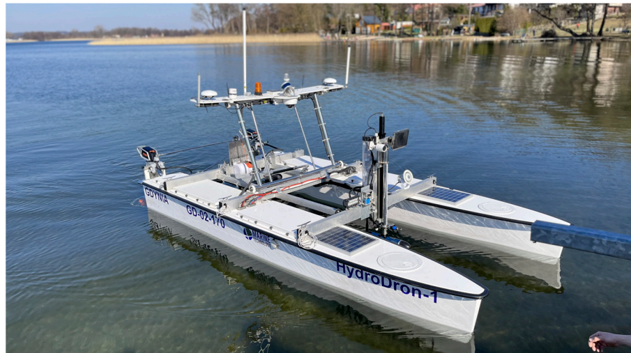
Figure 9. Autonomous survey vessel—HydroDron-1.
