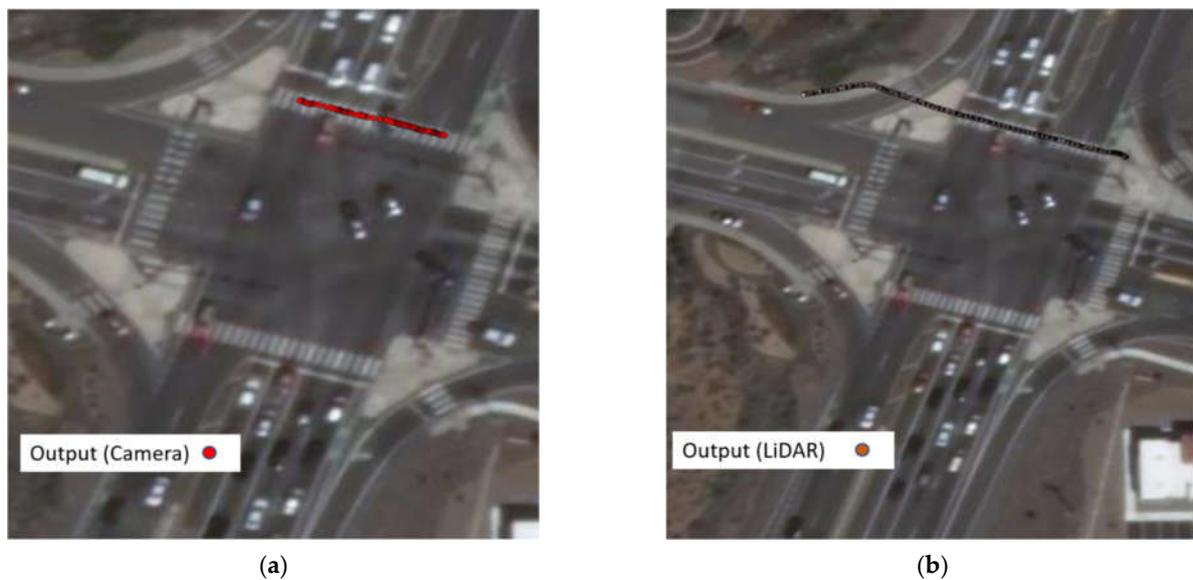
**Figure 17.** (a) Sample pedestrian trajectories captured by camera; (b) sample pedestrian trajectories captured by LiDAR.
