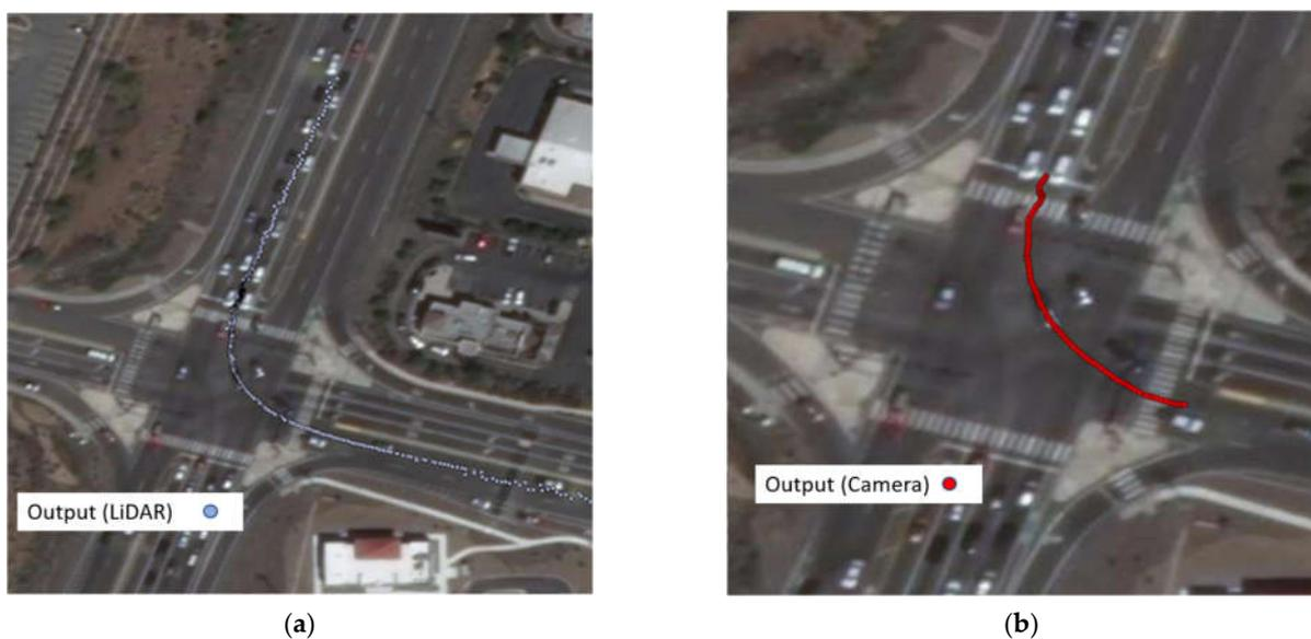
**Figure 13.** (a) Same vehicle trajectories captured by LiDAR; (b) same vehicle trajectories captured by computer vision.
