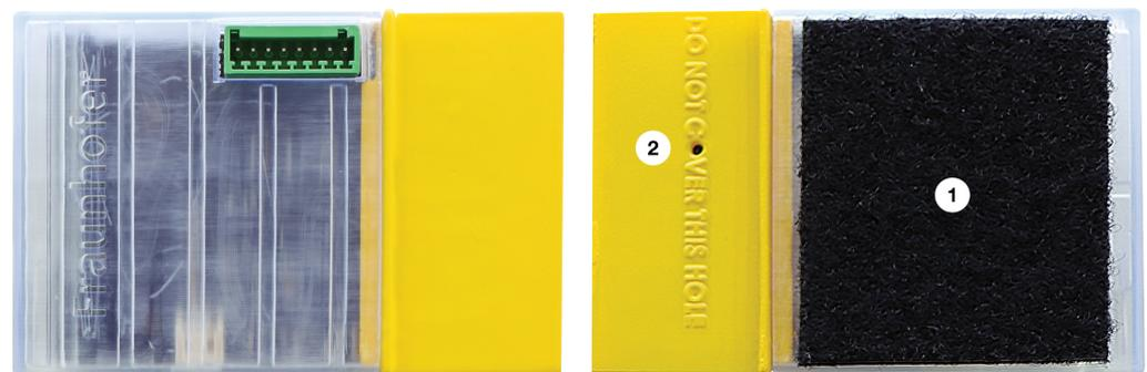
**Figure 4.** Three-dimensionally printed protective enclosure of the 5G IoT end device.
